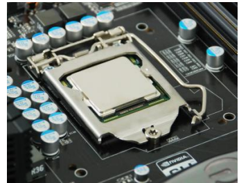
Align notches with notches on the CPU
