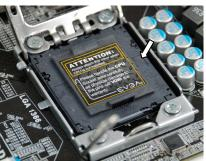
Note: Remove the process from its protective cover, making sure you hold it only by the edges. It is a good idea to save the cover so that whenever you remove the CPU you have a safe place to store it.
