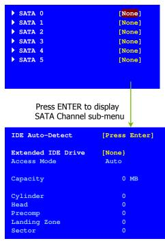
Press **Enter** to auto-detect IDE and SATA channels in the system. Once the channel is detected, the values for Capacity, Cylinder, Heads, Precomp, Landing Zone, and Sector are automatically filled in.
