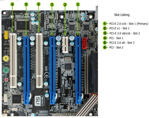
Note: When using 1 Graphic Card in PCI-E: Slot 1, a speed of x16 will be used. When using 2 Graphic Cards in PCI-E Slots: 1 and 3, a speed of x16/x16 will be used. When running 3 Graphic Cards in PCI-E Slots: 1, 3, and 5 a speed of x16/x8/x8 will be used.
