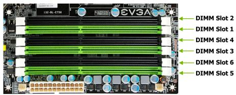
Use the following procedure to install memory DIMMs. Note that there is only one gap near the center of the DIMM slot. This slot matches the slot on the memory DIMM to ensure the component is installed properly.
