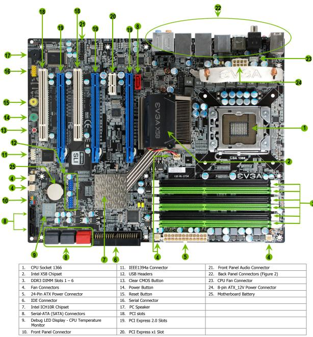
Figure 1. EVGA X58 SLI Motherboard Layout
