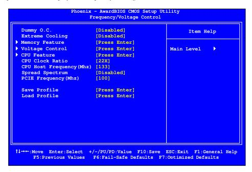
Figure 11. Frequency/Voltage Control Menu
