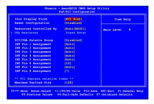
Figure 9. PnP/PCI Configuration Menu
