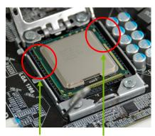
Align notches with notches on the CPU
