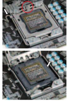
Note: Remove the process from its protective cover, making sure you hold it only by the edges. It is a good idea to save the cover so that whenever you remove the CPU you have a safe place to store it.
