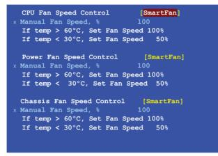
Use this menu to control the speed of the various fans on the motherboard. Set CPU fan speed to **[SmartFan]** when you want the speed of the fans automatically controlled based on temperature. To set the fan speed to a constant rate, select **[Manual]** and then enter the speed from 0% to 100%.
