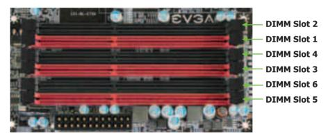
Use the following procedure to install memory DIMMs. Note that there is only one gap near the center of the DIMM slot. This slot matches the slot on the memory DIMM to ensure the component is installed properly.
