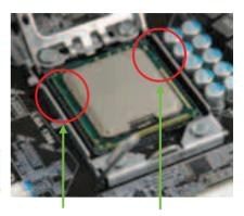
Align notches with notches on the CPU
