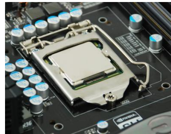
Align notches with notches on the CPU
